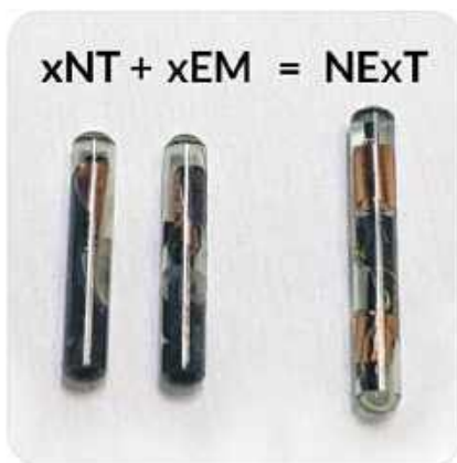
NExT RFID + NFC Chip Implant
