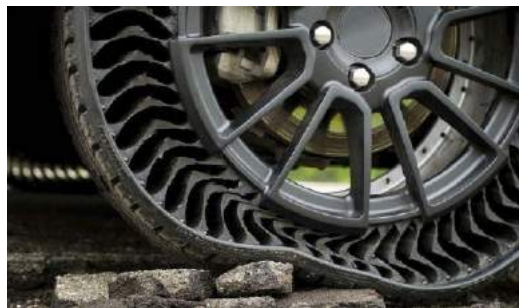
Michelin Uptis czyli Unique Puncture-proof Tire System
