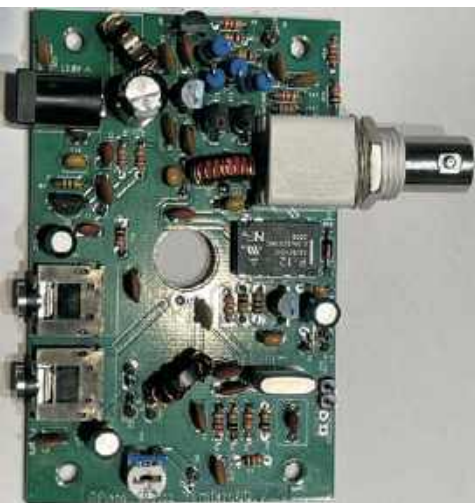
Transceiver mikroQ80 wg SP7NJ
