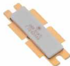
Tranzystor MRF 9180 (880 MHz, 170 W, 26 V)
