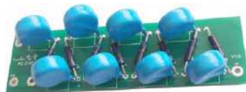
10. Generator Cockcrofta-Waltona AC-Z107 (© Alibaba)
