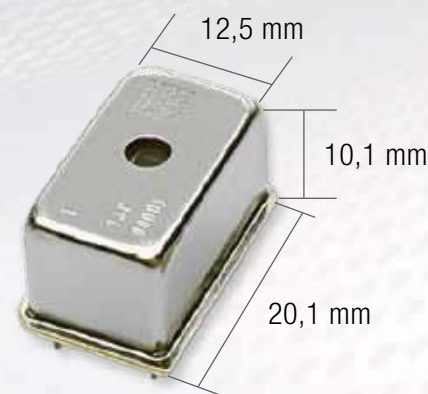
ultra-compact UV-mini-spectrometer C16767MA
