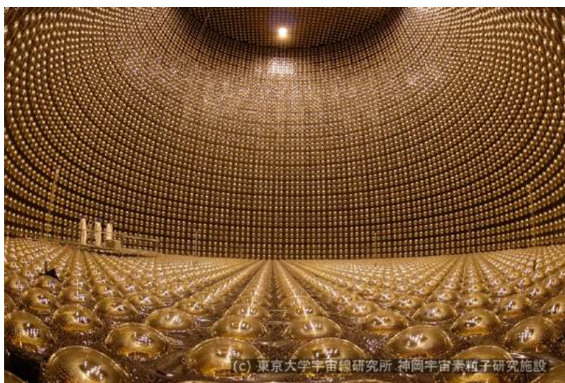
Rys. 3. Detektor neutrino w Kamiokande, Japonia. https://www-sk.icrr.u-tokyo.ac.jp/en/sk/experience/gallery/
